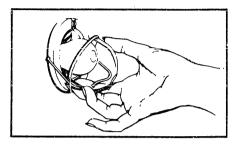
The oven lamp (bulb) is covered with a glass, removable cover which is held in place with a bail-shaped wire. Remove oven door, if desired, to reach cover easily.
